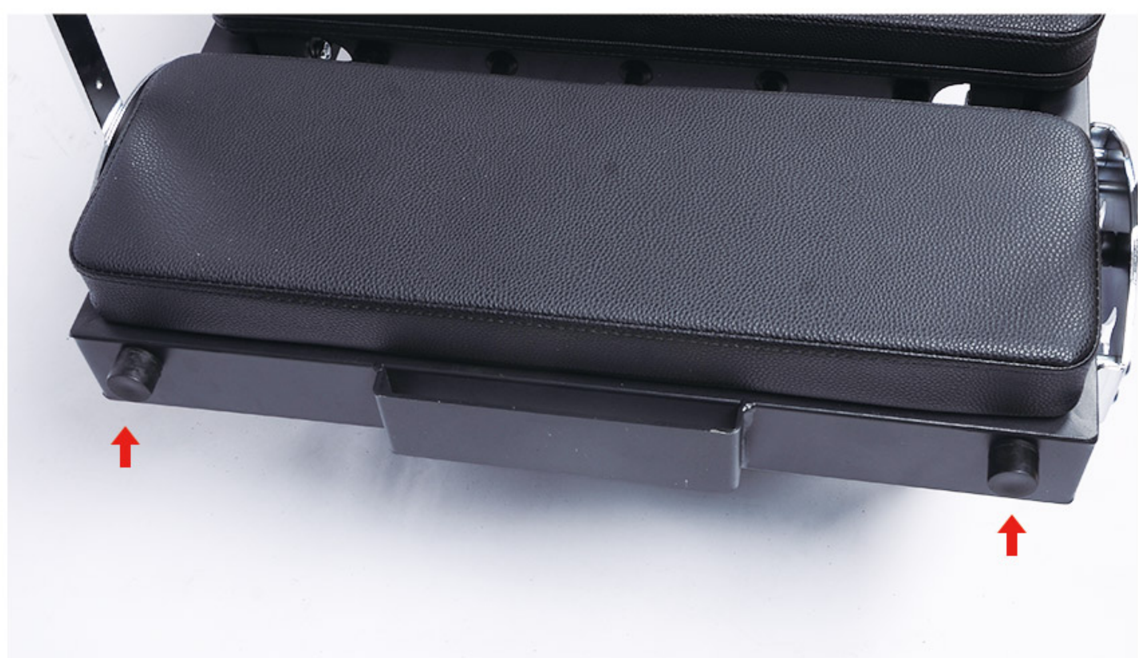
32. Insert the foot post into the hole on the other side and tighten it.
