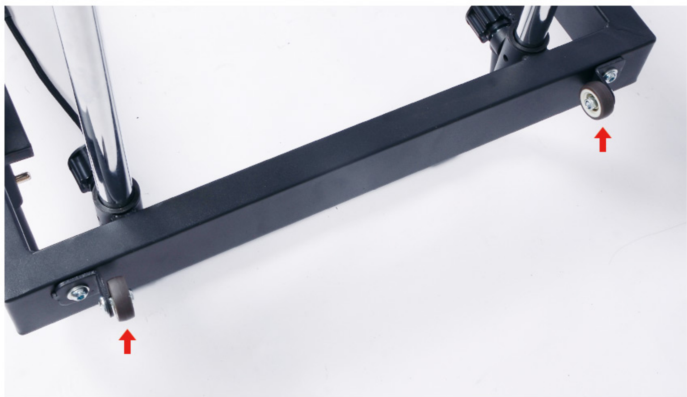
34. Follow the steps in Figure 33 to install the roller on the other side.
