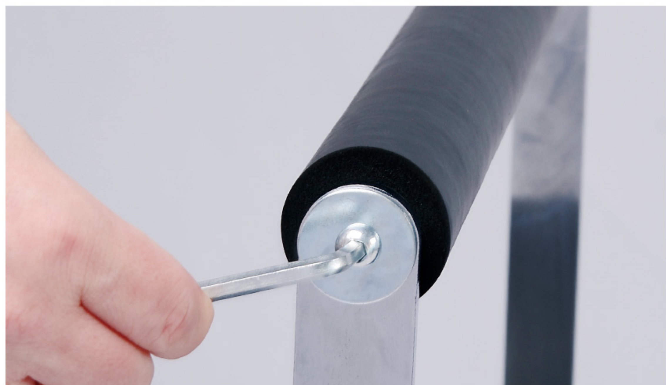
21. Tighten the for two sides gaskets and with an hexagon wrench.
